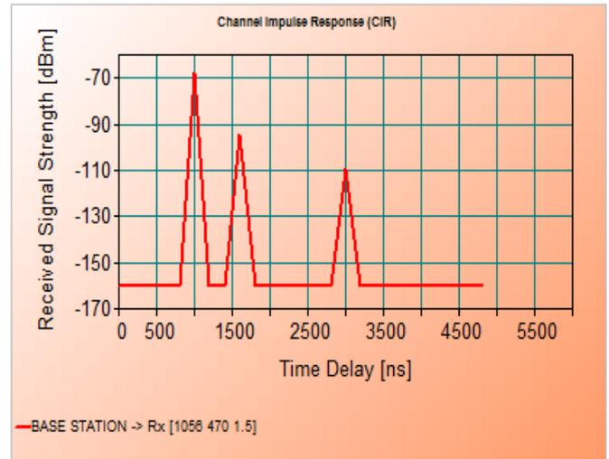
Figure 1: Channel Impulse Response at a Receiver Point
