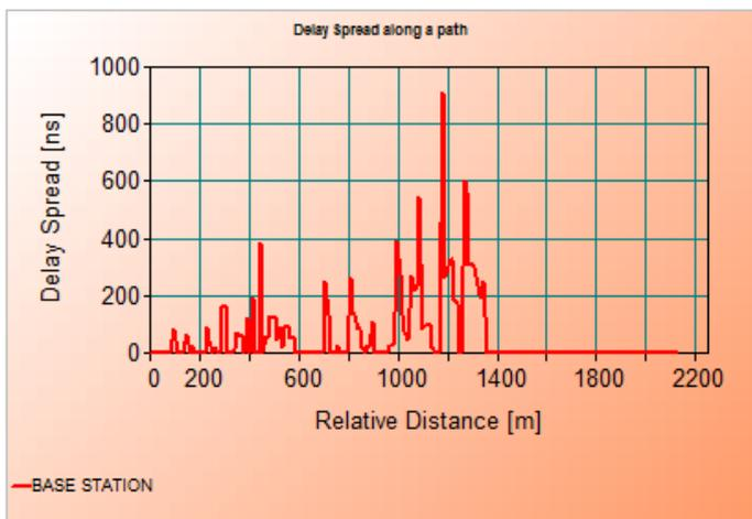
Figure 5: Delay Spread along the Path
