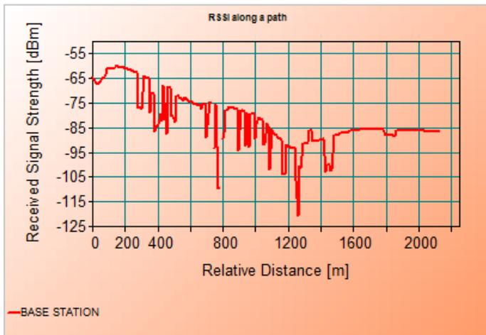
Figure 4: RSSI along the specified path
